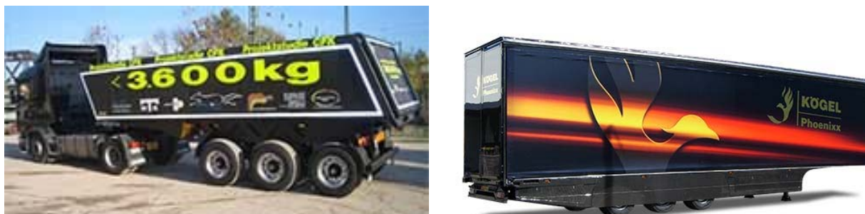
Figure 8. Low weight tipper with CFK body and CFK box body type semi-trailer
