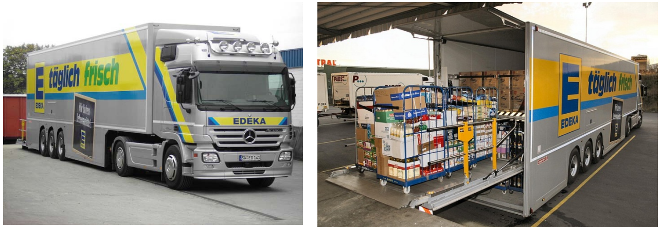
Figure 7. Two floor semitrailer with lift, 40 cm ground clearance and 4m box height, length 16.50 m, single wheel suspension on semitrailer for volume transports.
