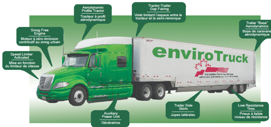
Figure 5. The Canadian “EnviroTruck” concept (2007) with fuel-reducing improvements.
